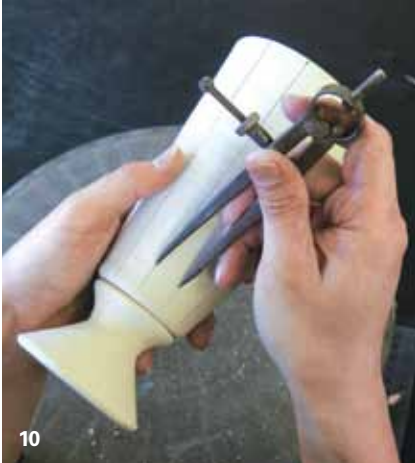
10 Measure the width between the vertical lines. Mark this measurement on the vertical line, then repeat the process.
