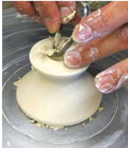
5 Trim the inside of the top of the stem to reduce thickness and weight.
