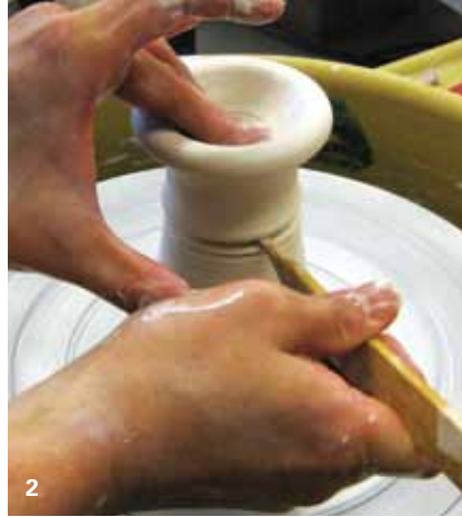
2 Use a wooden knife to make a cutting line for the stem.
