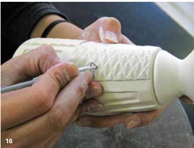
16 Refine the carved edges and add detailed carvings using a small triangular trimming tool.
