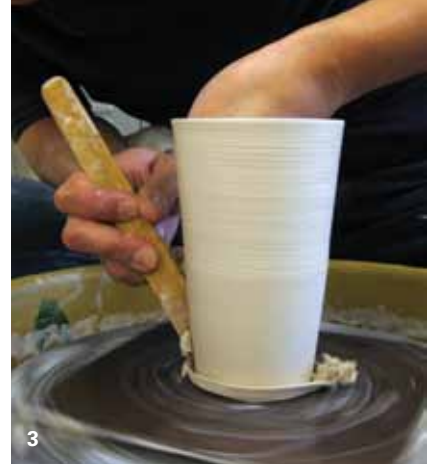
3 Use a wooden knife to trim down the bottom of the tumbler/body.
